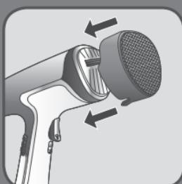
The steam cover filters water impurities and protects fabrics from water drips.
